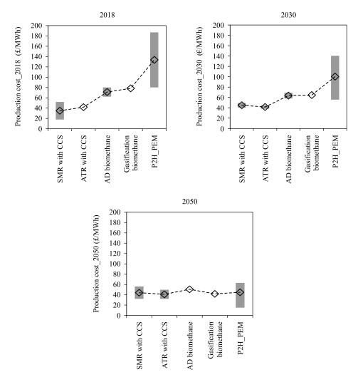
Fig. 5. Renewable gas production costs in 2018 and projections for 2030 and 2050.
